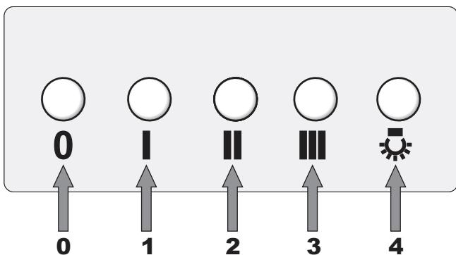
The button **4** is used to turn on and off the extraction hood lighting; independently of the engine work status, push this button to switch on/ off the lighting. The indicating light **8** turns on/off accordingly.
