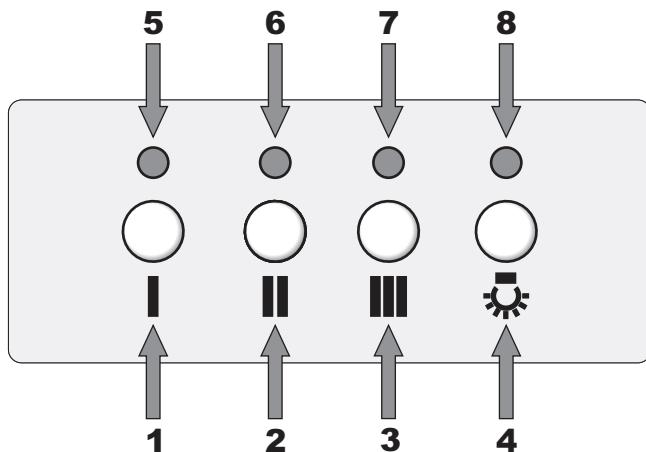
**Upper picture.** The buttons **1**, **2** and **3** serve the purpose of selection of the engine speed in range from 1 to 3.
