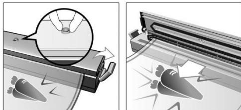
7. Pull the vacuum release valve in the middle of the cover.
