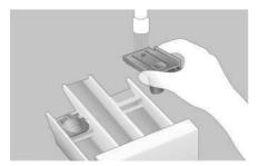
Clean the insert and the detergent chambers under running water.
