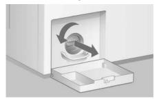
Unscrew the pump cover stepwise until the water starts draining out.
