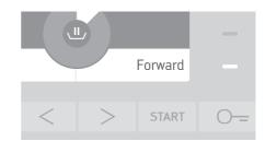
Press button Open the door O= (is not lit!). The programme will be interrupted and the door unlocked.
