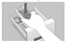
Replace the insert into the middle compartment.
