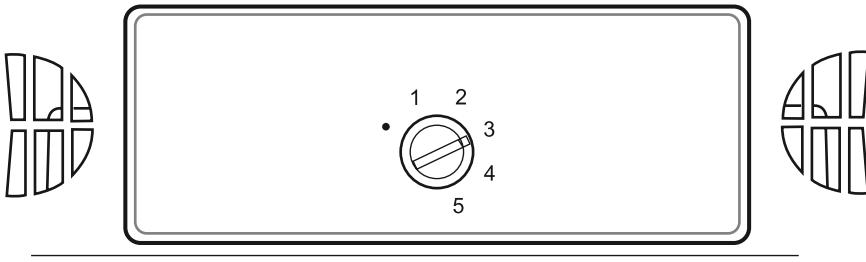
The thermostat automatically regulates the inside temperature of the refrigerator. By rotating the knob from position 1 to 5, colder temperatures can be obtained.
