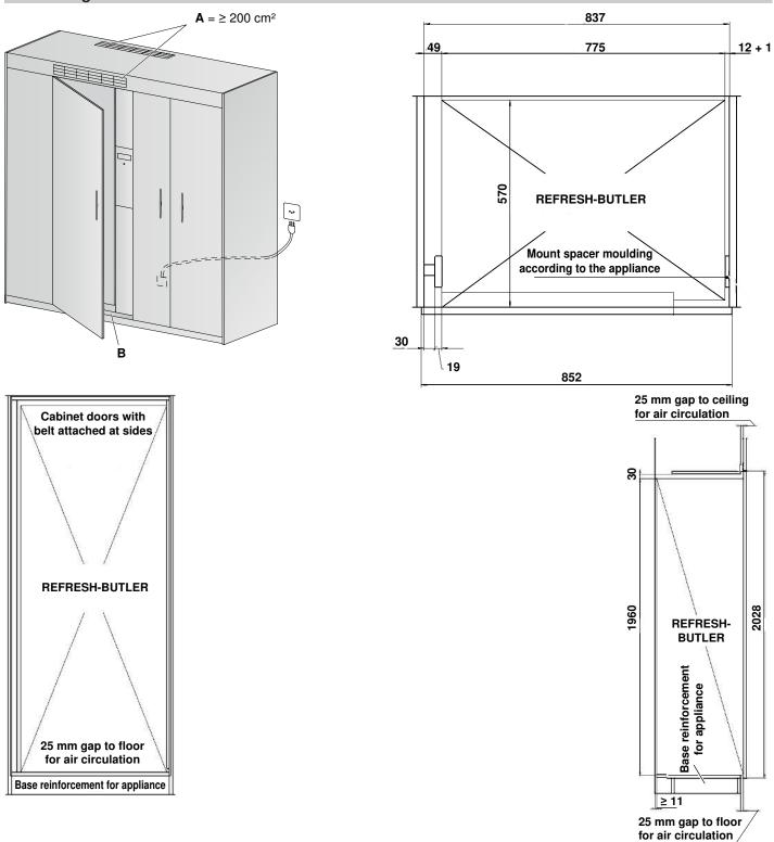
Ventilation slit on the top at the back or above the cab- B Load-bearing capacity of cabinet floor: min. 170 kg Α inet door
